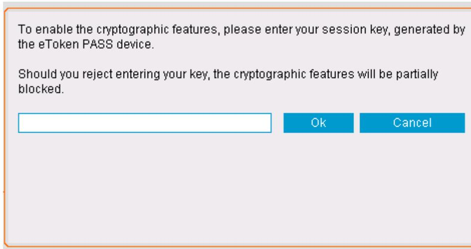
In order to generate the PIN code, press the button on eToken Pass. You will see the generated PIN code on the screen of the device. Type it in the entry line and press "Ok".
