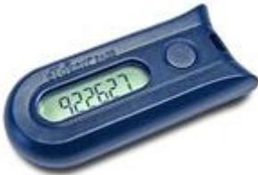
A special device is used for one-time password generation – an OTP-token. In the RB System of AO Mizuho Bank (Moscow), eToken PASS devices by Aladdin-RD are used.
